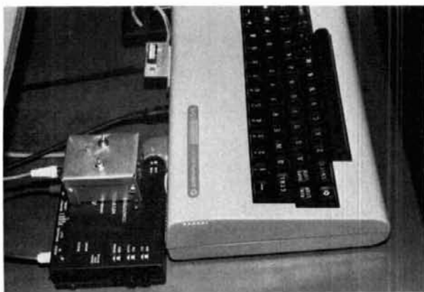
fig. 4. Prescaler mounted on MFJ interface.
